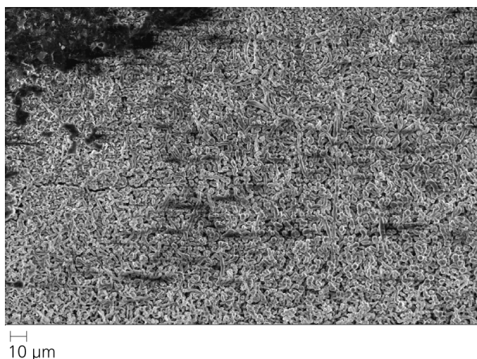
Figure 5.7: Ex-situ scanning electron microscope image of a cycled \text{SnO}_2 nanowire sample.
