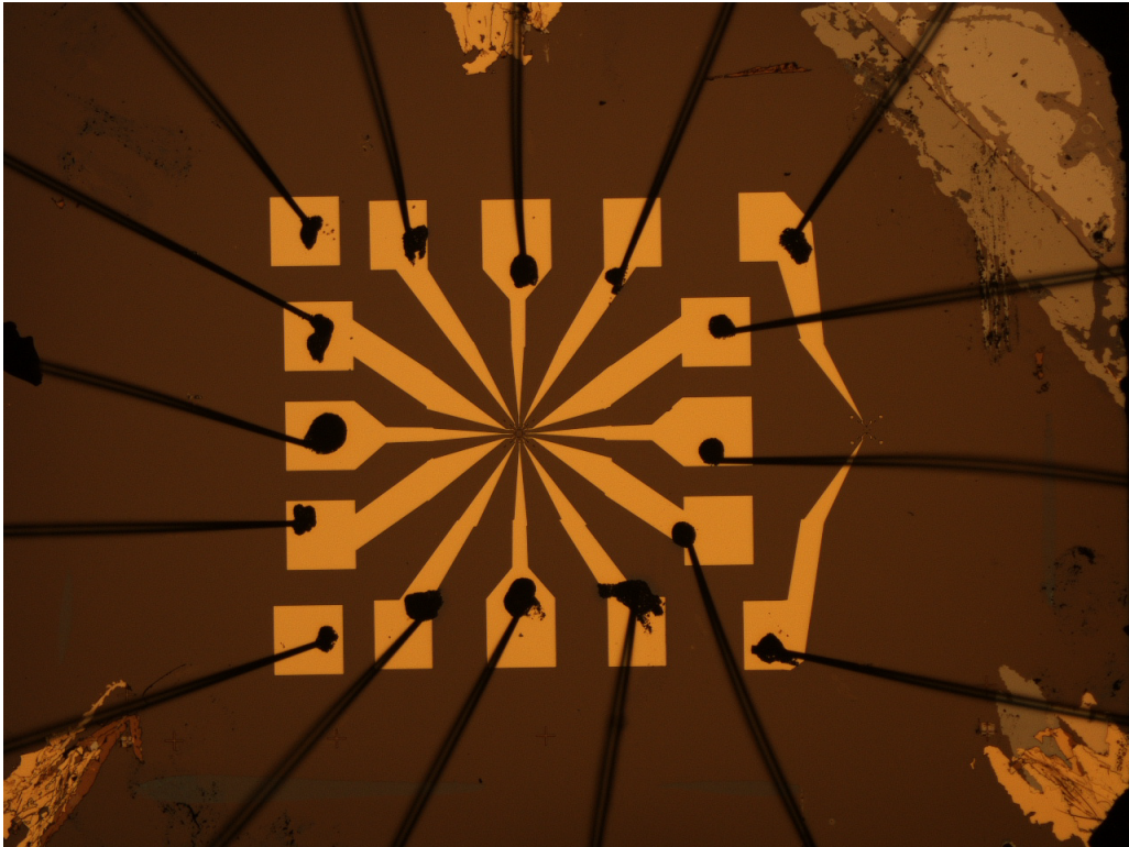
Figure 3.16: A picture of final sample, the sample is glue-bonded to chip carrier.
