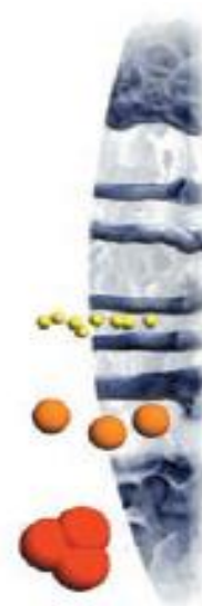
Figure 16 - Principle of size exclusion chromatography: Large proteins (red) do not intrude into the matrix, whereas smaller (yellow) and middle (orange) sized proteins can enter the pores and thereby elute later. (GEHealthcare)
