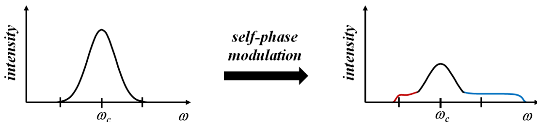
Figure 29 The Sketch indicates the frequency changes of an ultrafast light pulse experiencing self-phase modulation in combination with self-steepening with n_2 > 0 .
