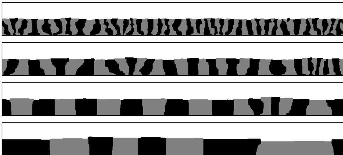
Figure 4.18: Surface snapshots at the end of simulation runs with NNN diffusion, E^{\text{AB}}/E^0 = 0.31 and F^{\text{A}} = F^{\text{B}} = 5 \times 10^{-3} \text{ ML s}^{-1} for T = 350 \text{ K} , 400 \text{ K} , 450 \text{ K} and 500 \text{ K} (top to bottom). The system size is 1024 \times 100 and the total coverage is \theta = 0.5 .
