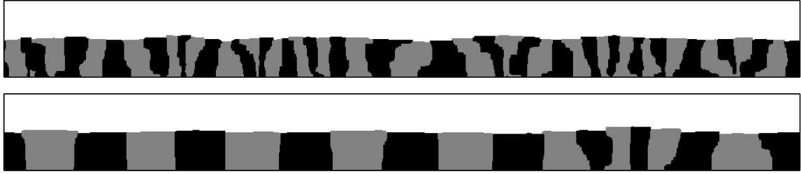
Figure 4.14: Surface snapshots at the end of simulation runs with NNN diffusion and T = 450 K. E^{\text{AB}}/E^0 = 0.51 (top) and E^{\text{AB}}/E^0 = 0.31 (bottom). The system size is 1024 \times 100 and the total coverage is \theta = 0.5 .
