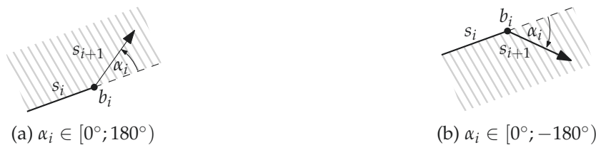
Figure 5.5: How we measure angles: angle \alpha_i is the angle between the straight line induced by s_i and s_{i+1} .
