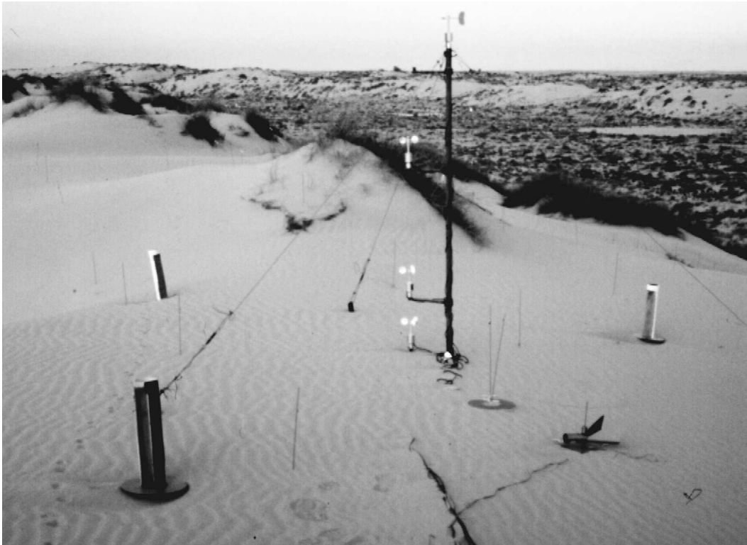
Figure 2.11: Instrumentation at site D, December 1998. Ripples and scour marks indicate recent sand transport by northerly winds. Also note accumulated organic litter in the lee of hummock N1 visible to left of the anemometer array.
