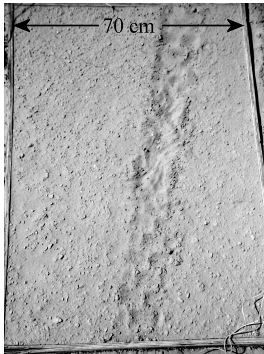
Figure 3.48: Surface crust sample after two years of development, 13/10/99. Note the motorcycle track running across.
