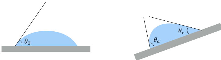
Figure 4.5: The schematic of equilibrium contact angle ( \theta_0 ) on a flat substrate, advancing ( \theta_a ) and receding ( \theta_r ) contact angles on an inclined substrate.
