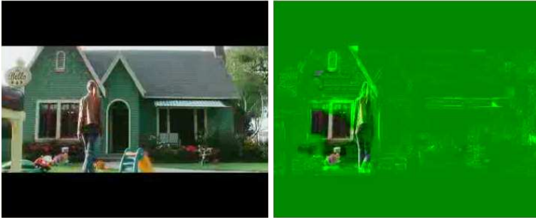
Figure 3.7: Distortion caused by lost I-Frame
