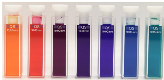
Figure 5. The optical properties of merocyanine dyes are easily modified by carefully adjusting the strength of the electron-rich and electron-poor end groups.
