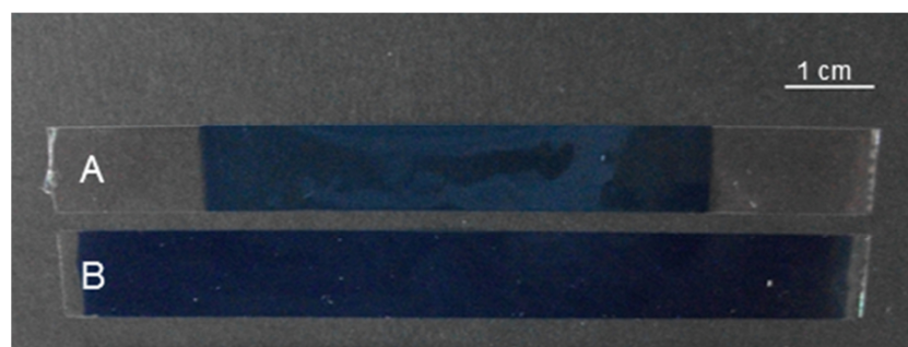
Figure 7.2 Photographic image of bilayers prepared with a 3 % (A) or 5 % (B) alginate solution cast on top of a PLA film.
