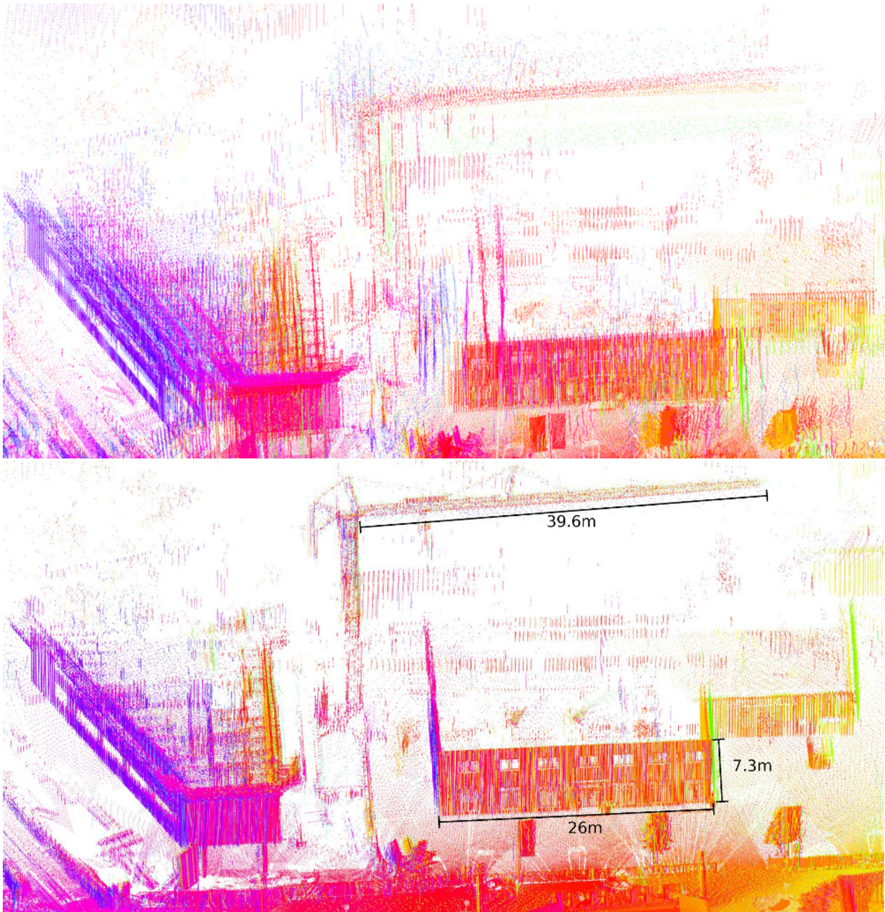
Figure 14. A more detailed view of the Salzburg dataset from Figure 13. The points are colored by their timestamps to provide contrast. The crane arm is approximately 42 m away from the trajectory. (Top) The initial point cloud. (Bottom) The optimized point cloud after processing with the semi-rigid registration algorithm.
