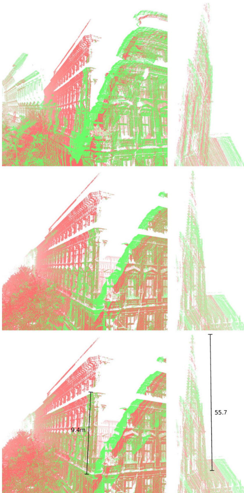
Figure 9. Close-ups of errors ( Top ), calibrated using the proposed algorithm ( Middle ) and the original, as calibrated by RIEGL Laser Measurement Systems ( Bottom ), Vienna dataset. ( Left ) Corner of a building. ( Right ) Top of church.
