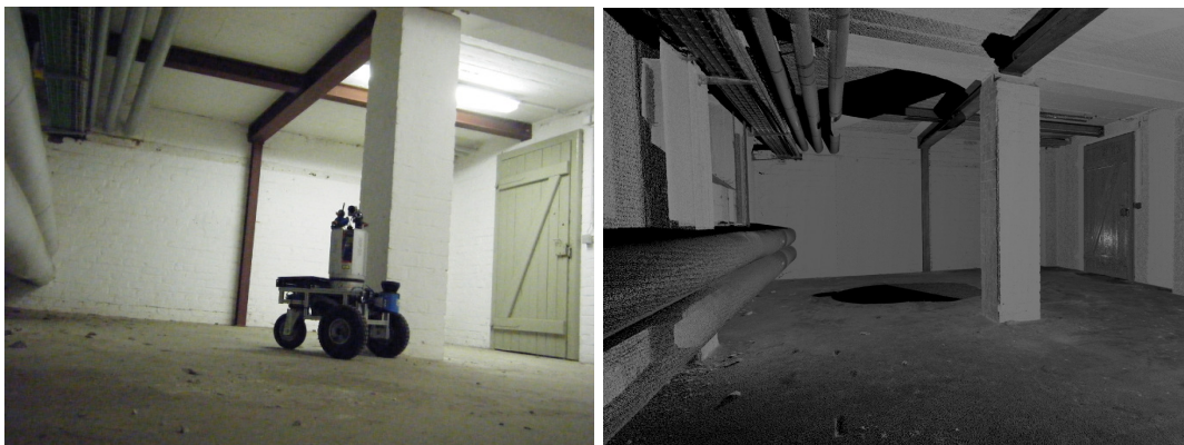
Figure 2. (Left) The robot Irma3D in the room where the experiments were carried out. (Right) The model of the basement (colored by reflectance) as acquired by standard terrestrial laser scanning.
