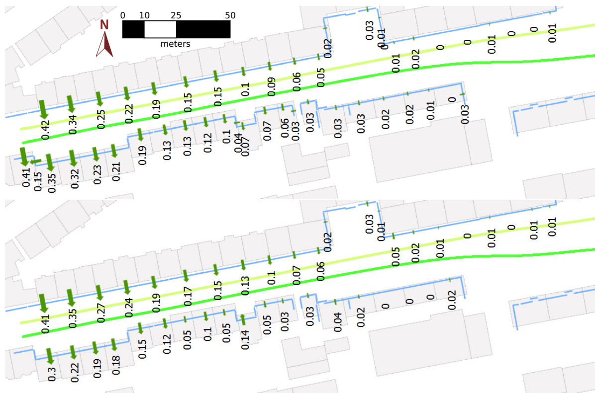
Figure 17. Facade errors with current state-of-the-art techniques in the Dortmund 2 dataset. From top to bottom: left sensor in the first pass compared to the left sensor in the second pass; left sensor in the first pass compared to the right sensor in the second pass; right sensor in the first pass compared to the left sensor in the second pass; right sensor in the first pass compared to the right sensor in the second pass.
