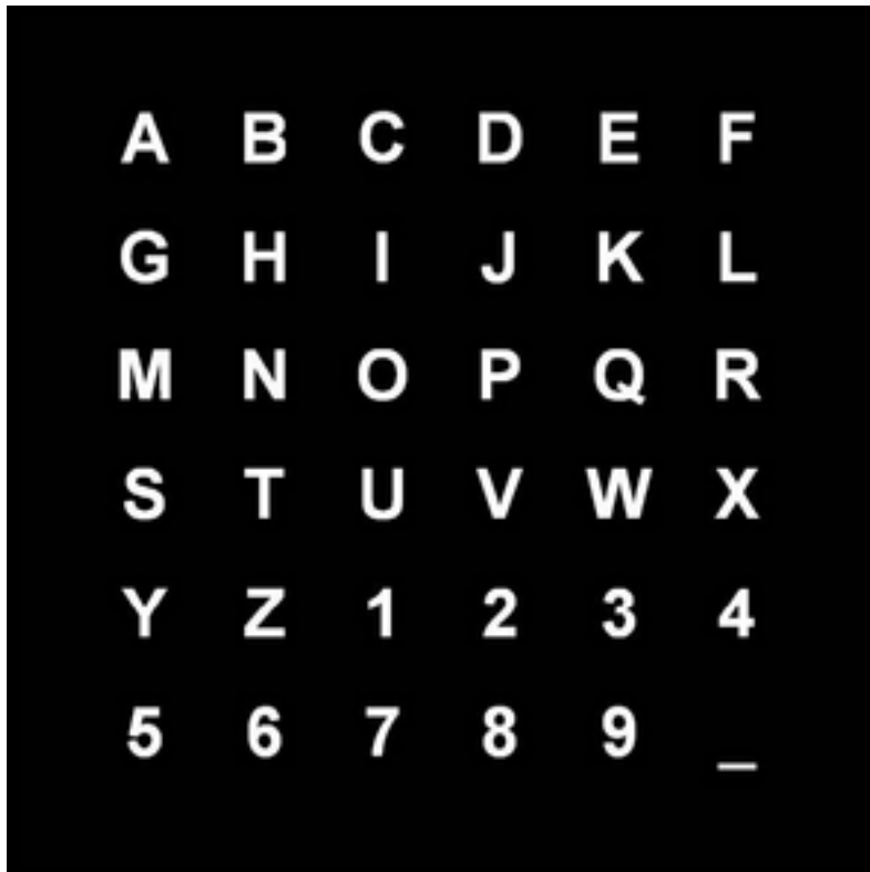
Figure 6: Matrix used for P300 based communication BCIs. Rows and columns are randomly highlighted while ERP responses are recorded. Only rows and columns containing the focused letter will elicit P300 responses, therefore identifying the chosen letter. Figure taken from Schalk & Mellinger, (2010).
