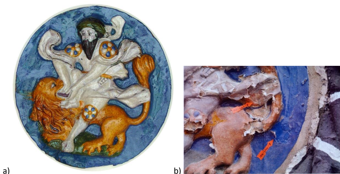
Figures 78 a and b: One of the restored medallions from the IHK-building in Lüneburg, Germany. Just restored (a; Furmanek, 2006) and six years after restoration (b, kindly provided by F. Schlütter). The arrows mark the points of sampling.
