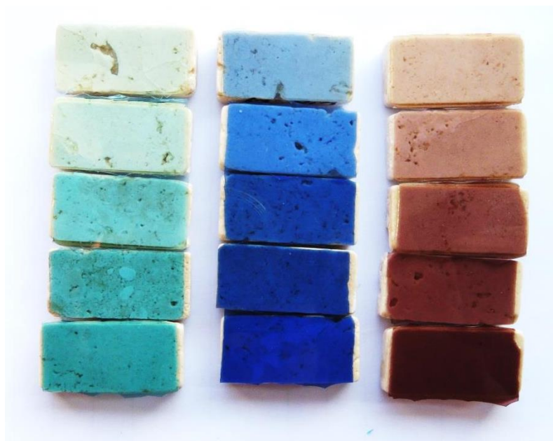
Figure 69: Glaze imitation samples with concentration series of CuO, CoO, and MnO 2 as colouring agents as given in table 23.
