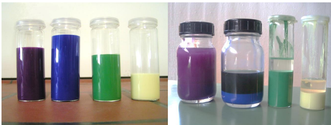
Figure 82 a) and b): Sedimentation behaviour of pigments manganese violet, cobalt blue, cobalt green and lead tin oxide yellow (from left to right) in ORMOCER® G after 187 h. The treatment with a roller mill and ultrasonic finger produces homogeneous compounds (a) whereas dispersion with a bead grinding mill leads to clearly visible sedimentation (b).
