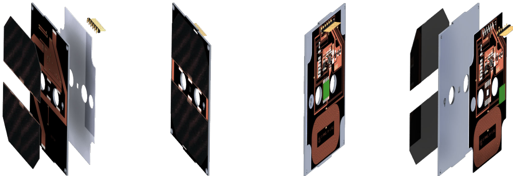
Figure 2.5: The side panels as a double layer PCB with aluminum core combine functions of structural stability, thermal balance, radiation protection, antenna ground plane, and electronics like wiring or sensor electronics in an integrated compact and lightweight design.
