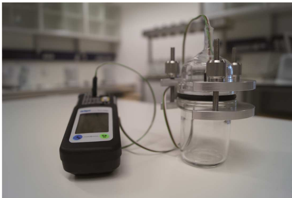
Supplementary Figure 3: Amperometric detection system for carbon monoxide.
