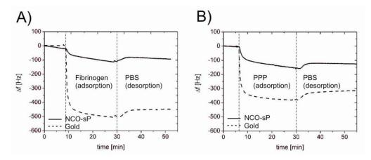
**Figure 2.** QCM frequency changes during protein adsorption measurements. NCO-sP(EO-*stat*-PO) coated and uncoated gold sensors were incubated in the QCM device with fibrinogen solution and 1 + 4 diluted human PPP (n = 3, for each Group). Differences between groups were calculated by univariate analysis of variance. Values of p < 0.05 were considered as significant and marked with \*.
