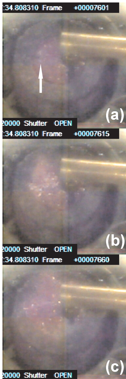
Figure 4.4: Frame of high-speed recording of an MFCI-run. 150 ml of tin melt were heated on 900 ° C. The frame rate was 20000 fps. At t = 0ms the water injection pump is started, after 100ms the solenoid opens and the video recording is started. It ends after t = 440ms and the trigger projectile is launched from the gun. 40.05 ms later it arrives at the melt surface ( t = 480.05ms , frame 7601, picture (a)). At t = 480.75ms (frame 7615) the melt surface breaks up, picture (b). At frame 7660 at t = 483.00ms (picture (c)) the recorded force signal in 4.3 (a) is maximum. Some ash particles leave the system around the injection tube. The attached video shows the complete process (see appendix E).
