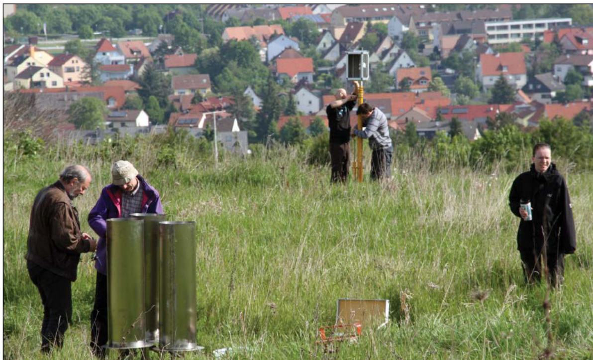
Fig. 2. Getting ready for the first experimental run: Scientists check the impulse cannons (left side in the foreground). An electrical field sensor is prepared by the team from the UK Met Office and National Centre for Atmospheric Science (right side in the background).
