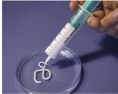
Figure 45: Ready-to-use CPC paste on the base of oil (Miglyol 812) (modified and reproduced from [273] with permission from Elsevier).
