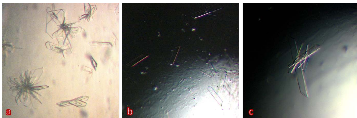
Figure 3.2-IV: Crystals of [saFabI·NADP + ·inhibitor] complexes: (a) [saFabI·NADP + ·55JS] grown in 100 mM Na/K-PO 4 , pH 6.5 and 32 % (v/v) MPD; (b) [saFabI·NADP + ·101JS] grown in 100 mM Na/K-PO 4 , pH 6.5 and 48 % (v/v) MPD; (c) [saFabI·NADP + ·101JS] grown in 100 mM Na/K-PO 4 , pH 6.5 and 46 % (v/v) MPD
