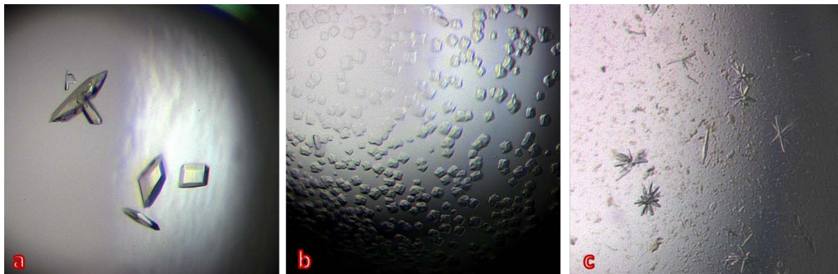
Figure 3.1-III: Crystals of [InhA·NAD + ·inhibitor] complexes: (a) [InhA·NAD + ·PT501] grown in 100 mM Tris/HCl, pH 9.0, 2.5 M NaCl; (b) [InhA·NAD + ·PT501] grown in 100 mM Hepes, pH 7.0, 3 M NaCl; (c) [InhA·NAD + ·PT511] grown in 3.5 M sodium acetate, pH 7.0 with a 1:100 PT501-seeding solution
