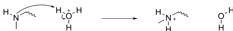
Figure 4.31: The acidic hydrolysis of amides is followed by a subsequent acid-base reaction removing \text{H}_3\text{O}^+ from the system.
