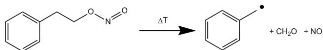
Fig. 2 The reaction scheme for the generation of benzyl radical by pyrolysis of 2-phenylethyl nitrite.
