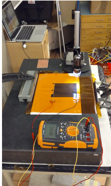
Figure 5.2: Set-up of the mechanical stretching test of the Kapton ® substrates.
