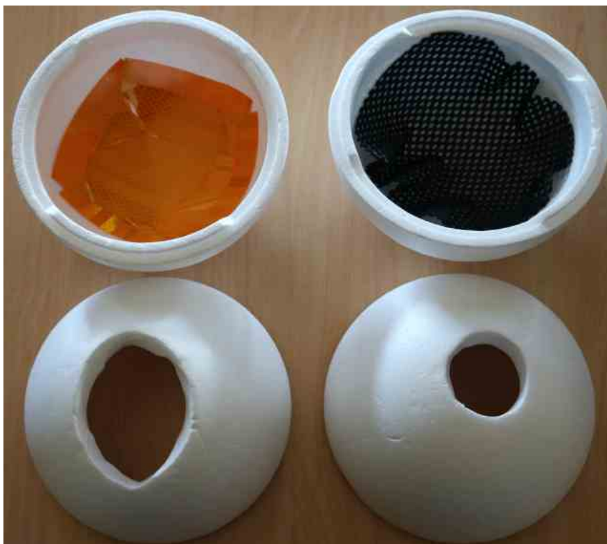
Figure 8: Eye models. Left: cat's eye with reflective tape, right: human eye (picture taken by Sabine Glaab)
