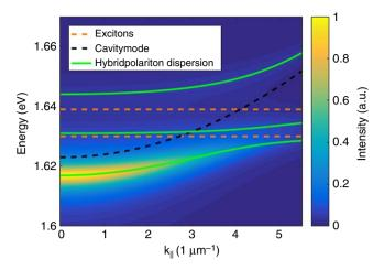
**Fig. 5** Simulated hybrid polariton dispersions of the Tamm device. Occupation numbers of the hybrid polariton states at 140 K are obtained using a thermodynamical approach. The parameters used for the simulation are obtained from fitting the data shown in Fig. 4d with the coupled oscillator model. The colour coding is the same as used before
