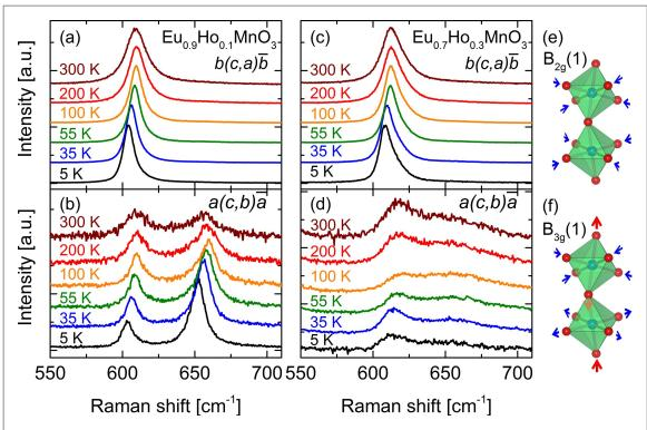
Figure 1. Temperature-dependent polarized Raman spectra for ((a) and (b))  $Eu_{0.9} Ho_{0.1}MnO_3$  and ((c) and (d))  $Eu_{0.7} Ho_{0.3}MnO_3$ . The spectral range comprises the octrahedron breathing modes  $B_{2g}(1)$  ( $\approx$ 610 cm $^{-1}$ ) and  $B_{3g}(1)$  ( $\approx$ 660 cm $^{-1}$ ). ((e) and (f)) octahedron elongation patterns for  $B_{2g}(1)$  (e) and  $B_{3g}(1)$  (f).
