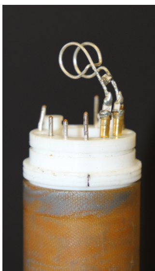
Data 10.5: Technical information of the ^1\text{H} 5 mm Helmholtz coil
