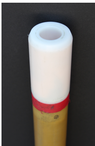
Data 10.8: Technical information of the ^1\text{H} 20 mm birdcage coil
