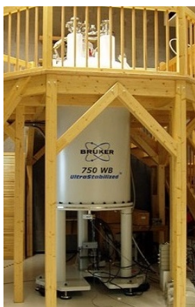
Data 10.2: Technical information of the Bruker Avance 750 WB in Würzburg
