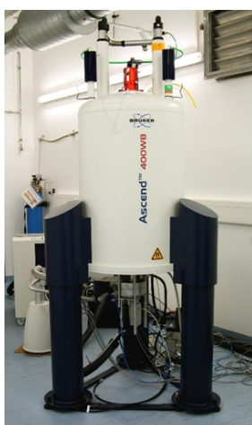
Data 10.4: Technical information of the Bruker Avance III HD 400 WB at IPK Gatersleben
