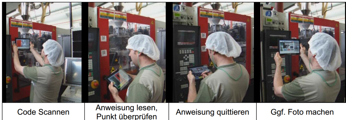
Figure 5.34: “Visual Control” function for supporting maintenance tasks (see [138])
