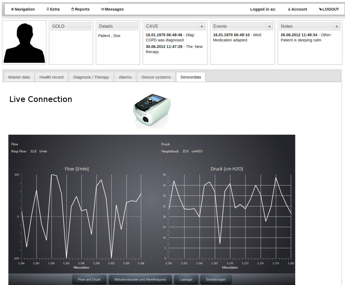
Figure 4.19: Lower part the telemedical work place showing the integration of the Java applet for remote operation of a flow generator.
