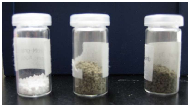
Fig. 85: Cerasorb ® particles made from calciumapatite (left), Cerasorb with physisorbed nanodiamond with a concentration of 4% wt (Diasorb ® , centre) and Cerasorb with physisorbed nanodiamond with a concentration of 8% wt (Diasorb ® , right).
