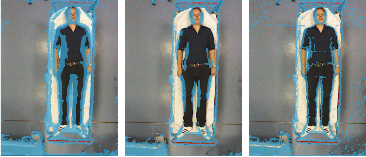
(a) Threshold of 40^\circ , normal smoothing size factor of 15 (b) Threshold of 60^\circ , normal smoothing size factor of 15 (c) Threshold of 60^\circ , normal smoothing size factor of 5
