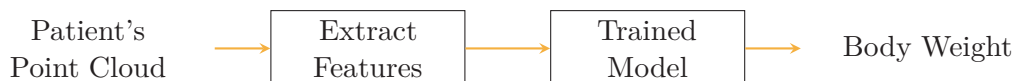
Figure 5.1: Process of body weight estimation: Based on the previously segmented point cloud features are calculated. Those features are forwarded to an ANN.
