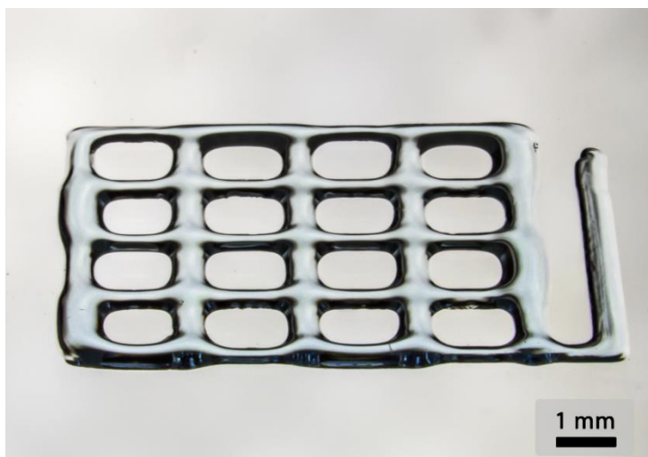
Fig. 4.29| Light microscope image of a printed construct composed of orthogonal stacks of hydrogel strands with a base area of 12 x 12 mm 2 and a strand-center to strand-center distance of 3mm.
