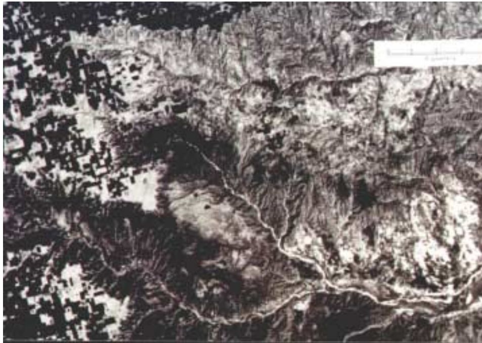
Figure 14. LANDSAT imagery from 1978 for the determination of eolian deposits in light gray.
