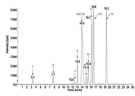
Figure 1: HPLC chromatogram of mercapturic acid standards with 5  $\mu$ g/ml CH<sub>3</sub>OH/H<sub>2</sub>O (1:2 v/v) each, obtained with CNL 129 Da survey scan on a Reprosil Pur AQ column with optimized HPLC gradient. Assignment of each peak (no. 1-13) is given in Table 9.
