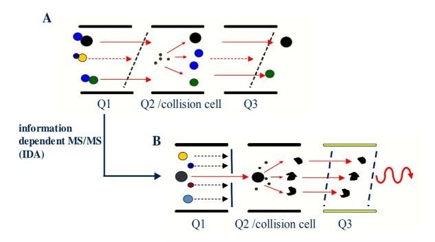
Scheme 6: Scheme of the scanning series of an IDA method, combining a constant neutral loss survey scan (A) with an enhanced product ion (EPI) scan, using a linear ion trap (B). Q1, Q2, and Q3 describe the quadrupoles for ion transport and filtering, wheras Q2 serves as collision cell (nitrogen as collision gas (•)) in both scan modes. In (B), Q3 is used as a linear ion trap to collect fragment ions generated by Q2.
