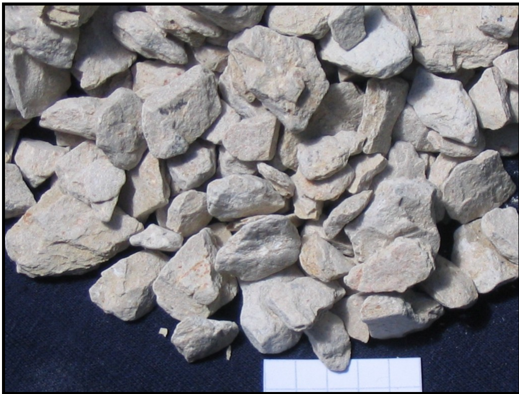
Fig. 3.18: Whitish to light bluish-grey weathered pieces of bentonite from the DIBA Tuff. Scale is 5 cm in length.
