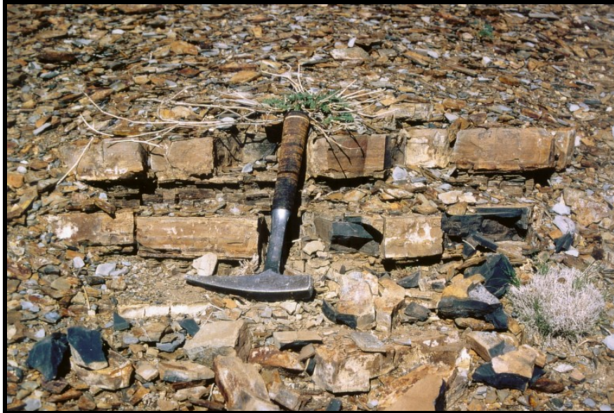
Fig. 3.43: Black, carbonaceous, dolomitic limestone layer of the so-called Goris Limestone Beds in the upper part of the Whitehill Formation at the Eisenstein locality.
