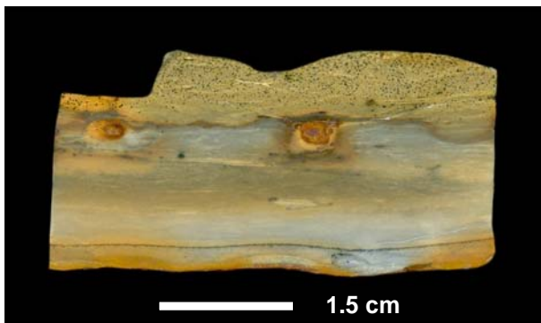
Fig. 3.37: Panorama Tuff 1: Polished section of the light weathering, chert-like, albitized and silicified zone along a tuffaceous horizon within bluish-greenish-grey, peppered shales of the Whitehill Fm. (Panorama facies succession). The brownish spots at the top of the layer most probably represent hematite-goethite pseudomorphs after pyrite. This layer is equivalent to that of the Khabus locality (see Fig. 3.36 & 3.39).
