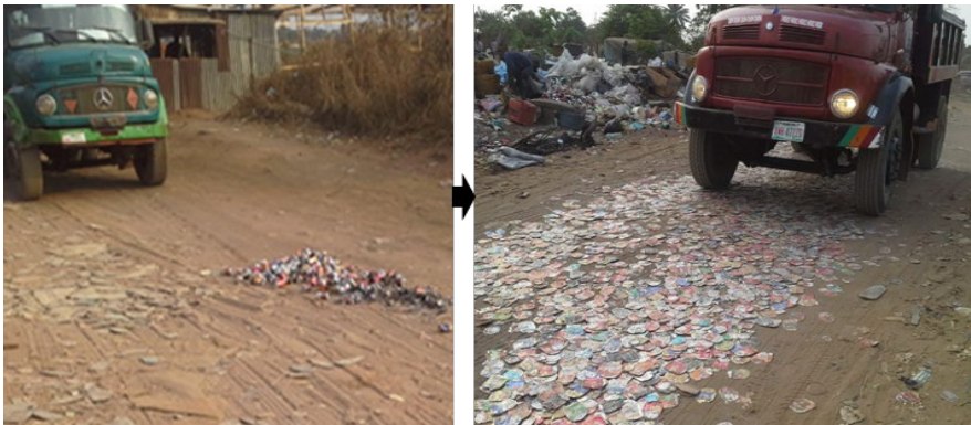
Figure 4.22c Compression of empty gathered cans by waste sorters before selling. (Photos Ache, 09.02.2017).
