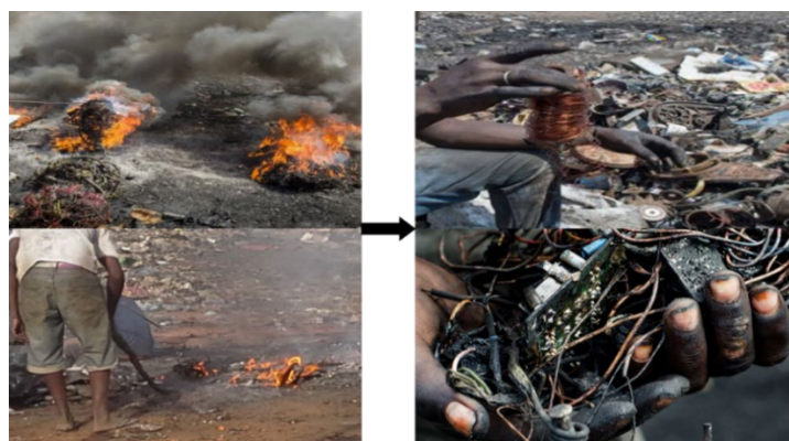
Figure 4.22b Burning to retrieve copper/brass from E-waste (Notice the fingers are damaged from burning and sorting) (Photos Ache, 09.02.2017).
