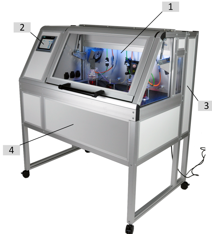
Figure 3.2: A tailor-made incubator system was constructed to provide appropriate culture conditions for hiPSC suspension cultures. In addition, the incubator system contains all equipment necessary for automated process control and monitoring. Suspension culture vessels were placed freely within the incubated space (1). The incubator atmosphere, liquid-handling devices, stirrer agitation speed and data management was accessed via human machine interface (2). The process control equipment and sensor transmitters were located in the rear compartment of the incubator (3). The in situ imaging microscope was incorporated into the lower cabinet beneath the incubation area (4).
