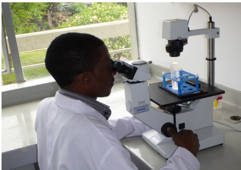
Photograph 1: Analysis of the modified Harada Mori culture tubes with an inverted microscope
