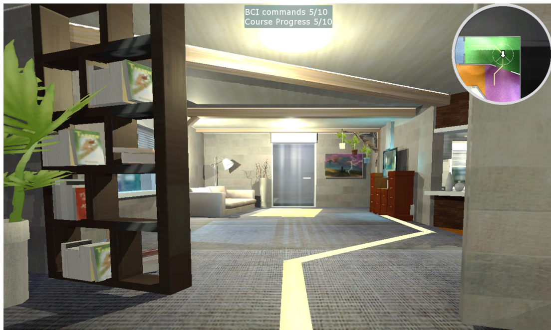
Figure 10.1: Updated environment for guided navigation. A line on the floor in front of the user indicates the required course. Numbers on the top of the screen show the total number of commands received and the total number of correct commands.
