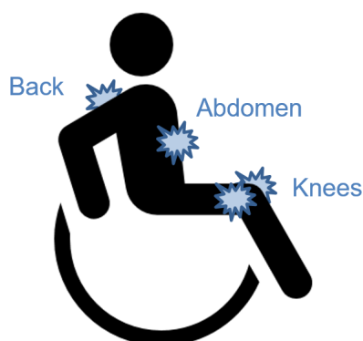
Figure 7.1: Schematic of tactor positions on a potential user. Positions at the abdomen, back, left and right knees encoded the movement commands forward , backward , left and right turn , respectively.
