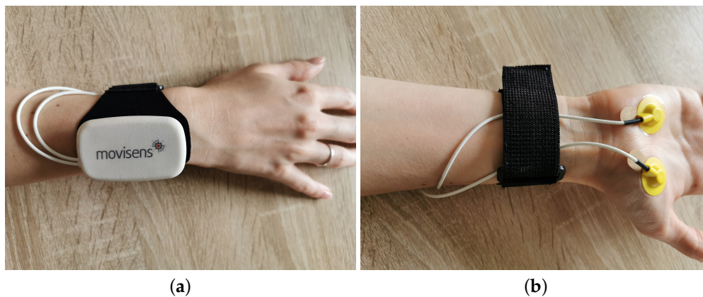
Figure 3. Attachment of the sensor EdaMove 3. (a) Top side of the EdaMove 3 sensor; (b) Electrodes attached to the palm.
