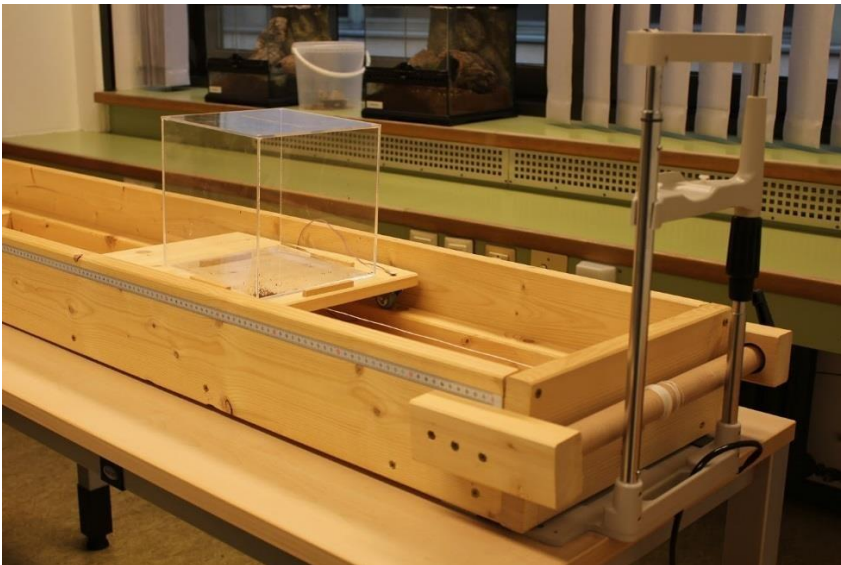
Figure 2. Setup for BAT. The spider is placed in the plastic box, which is then placed on a movable platform.
