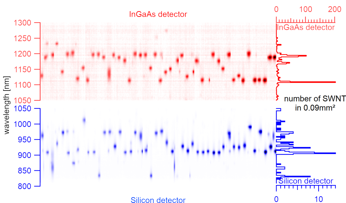
Fig. 51: The exact scan technique is a scan along the trench. Eleven spectra are taken around a rough position with the goal of identifying the exact location of the single-wall carbon nanotube from the image. The scan in this image is ordered by the intensity with features of the highest intensity located on the right side.
