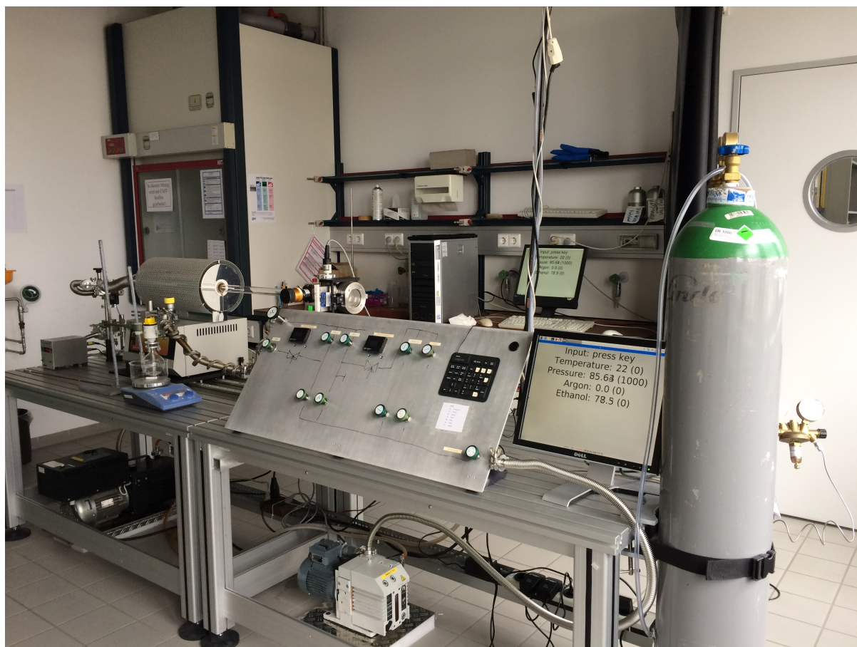
Fig. 12: The Chemical Vapor Deposition Reactor consists of an oven in the center of the image and a gas control with different inlets on the right. The pump at the left can achieve constant flow synthesis at 10mbar. The quartz tube connects the gas inlet and pump and allows temperatures of 800°C.
