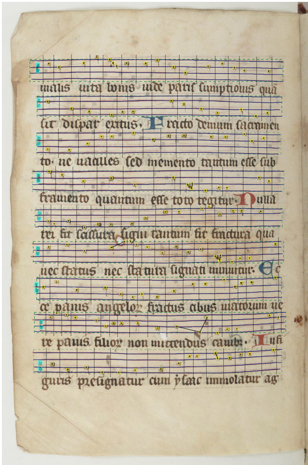
Figure 13. The page visualises the full prediction of the staff line and symbol detection. Encoded staff lines are drawn as blue lines on top of the red staff lines of the original manuscript, the green dashed lines mark the bounding boxes of single staves. The vertical dashed lines separate neumes whose NCs are drawn as yellow boxes. Graphical connection with a neume are indicated by a black stroke between two NCs. The reading order is represented by a thin dotted line that connects all NCs withing a staff. Small crosses inside of the yellow box of a NCs mark the discrete location of the symbol relative to the staff lines. The cyan symbols mark clefs.
