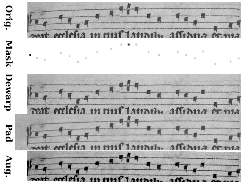
Figure 7. The first line shows the cut off original input image. The next one is the target mask for the FCN in which notes and clefs are marked. The next three lines show the dewarped, padded and an augmented version of the original image.
