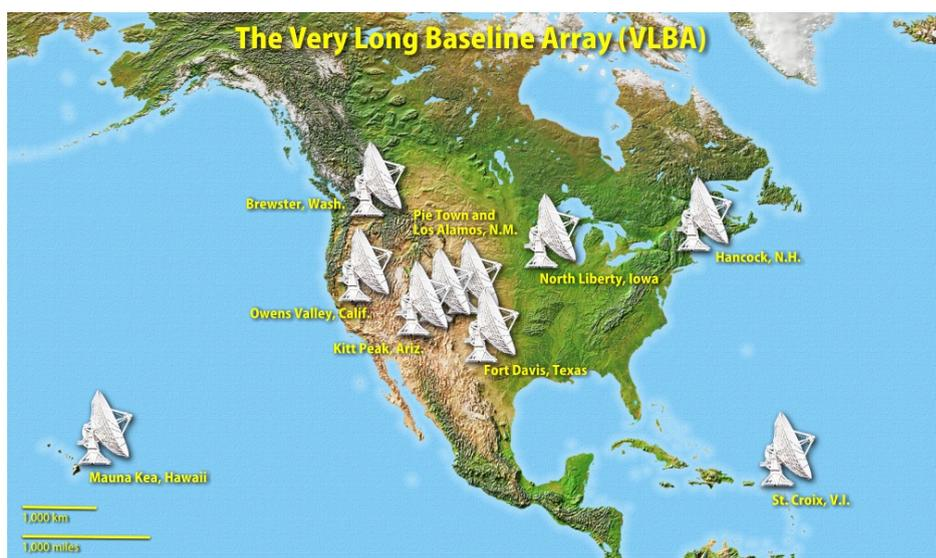
Figure 2.1: The Very Long Baseline Array operates on the principle of Very Long Baseline Interferometry (VLBI). This giant radio interferometer has a detectable frequency range of 1.2 GHz to 96 GHz. Image from [30].
