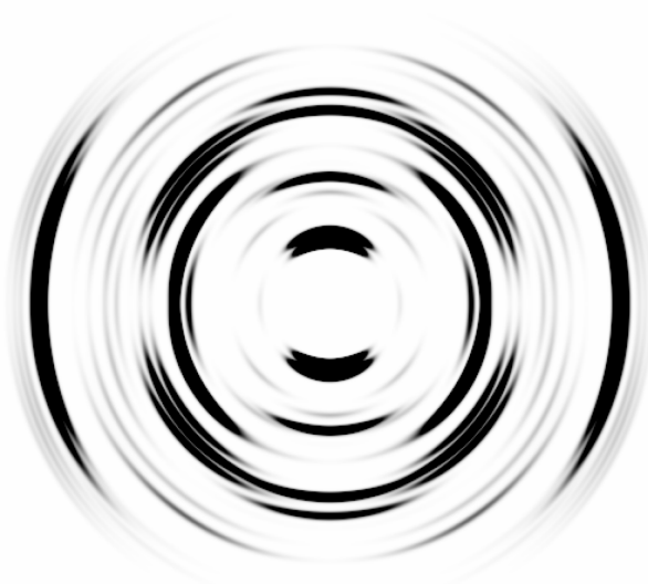
Figure A93. Diffraction pattern as simulated with CLEARER for the Col r phase of DPP 2 .
