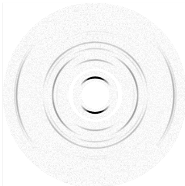
Figure A94. Diffraction pattern as simulated with CLEARER for the Col h phase of DPP 2 .
