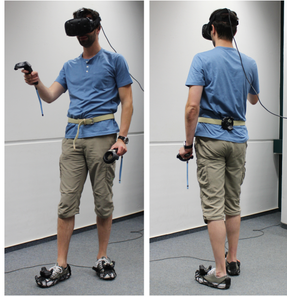
Figure 5: Virtual bodies are implemented by tracking the positions and orientations of feet, back, head and hands.
