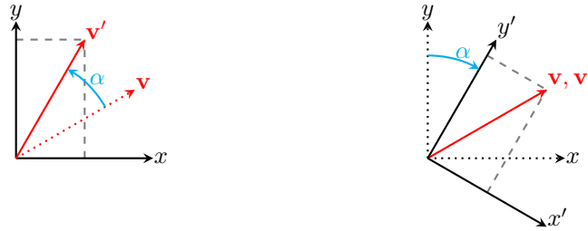
FIGURE 3.1: Active rotation (left) and passive rotation (right) around an angle \alpha . The sign of \alpha changes depending on the type of rotation.
