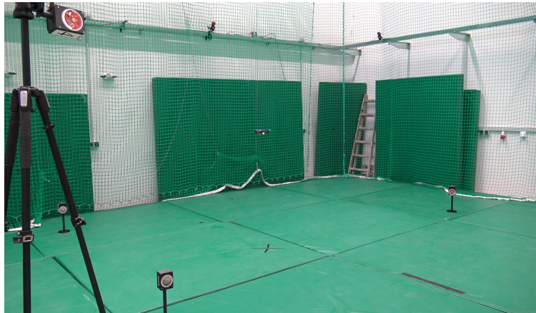
FIGURE 2.41: LPS based on UWB anchors and DS-TWR.
