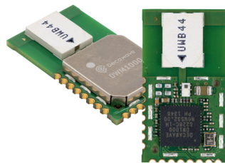
FIGURE 2.32: DecaWave UWB module DWM1000 [116].
