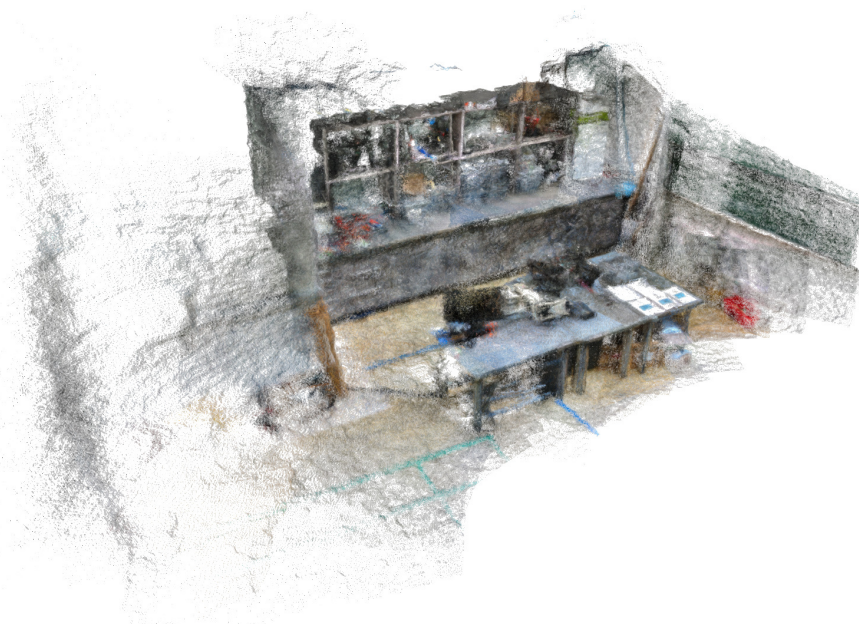
FIGURE 7.3: 3D map of the drone laboratory.
