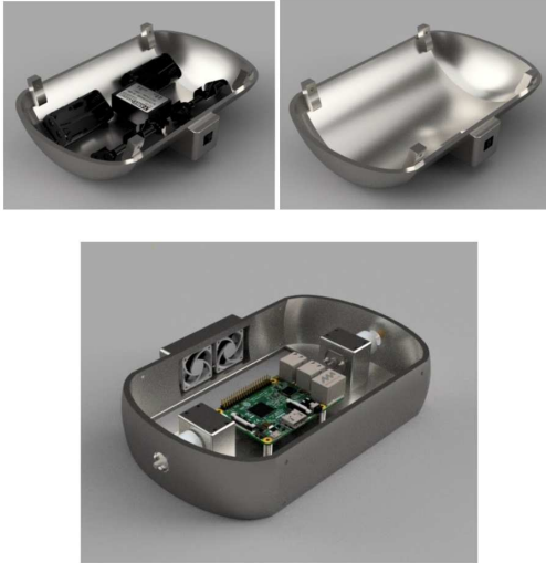
Figure 3.2: The top left image demonstrates the bottom segment of the robot. The top right image shows the top segment of the robot and the bottom image shows the middle segment of the robot.
