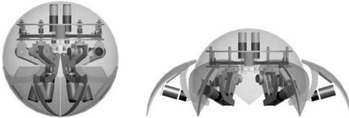
Figure 7.30: Hybrid Hex-A-Ball spherical robot with walking and climbing locomotion [119].
