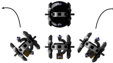
Figure 6.22: Changing the weight distribution by changing the pose of the battery leads to a curved path.
