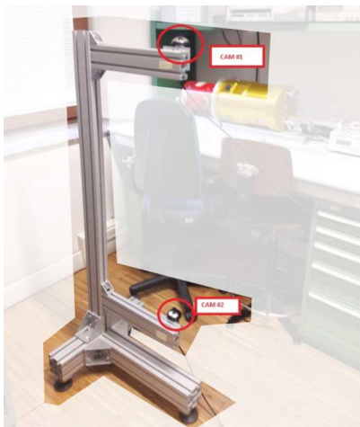
Figure 3.21: Laboratory set-up simulating the stereo block with panoramic cameras. In red the two optical heads.
