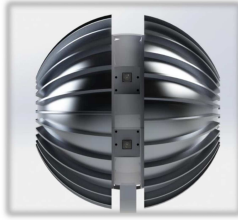
Figure 7.26: A differential driven robot developed with two individually operated wheels [122].
