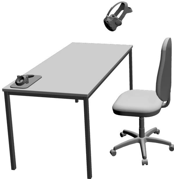
Figure 3.2: Apparatus. Participants sat in front of a table. They wore a head-mounted display. Participants looked at a virtual representation of the table. Meanwhile, they touched the real table. A sensor tracked the position of the table.
