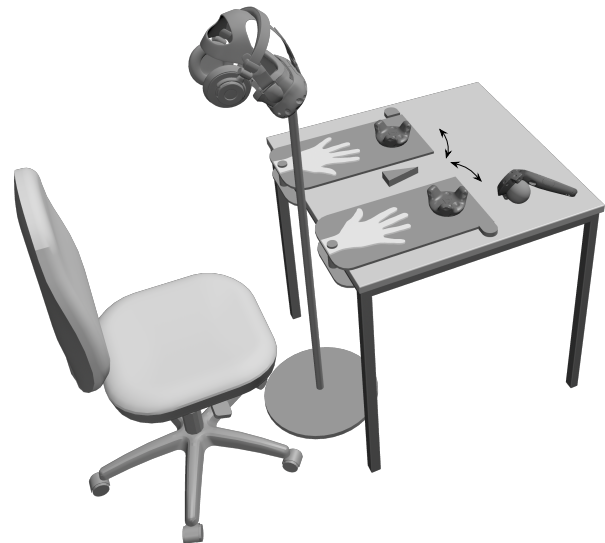
Figure 6.2: Apparatus. We presented visual stimuli in a immovable head-mounted display. Participants placed their hands on two hand rests. The experimenter delivered visuotactile stimulation with a styrofoam ball attached to a position sensor. The experimenter delivered visuomotor stimulation by rotating the hand rests. Sensors tracked the position of the hand rests. We presented Brownian noise in headphones.
