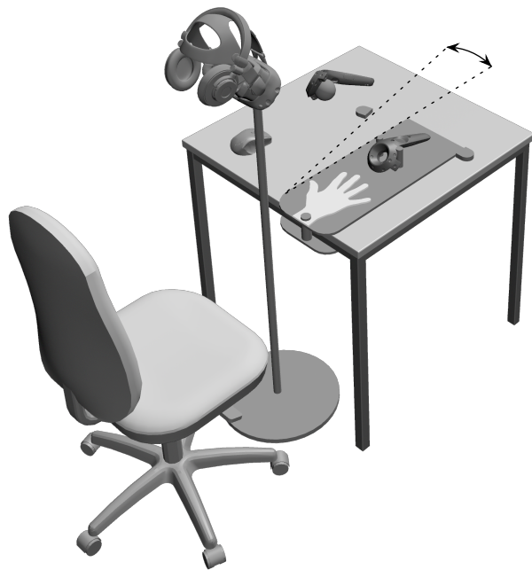
Figure 4.2: Apparatus. We presented visual stimuli in an immovable head-mounted display. Participants placed their right hands on a hand rest. The experimenter delivered visuotactile stimulation with a styrofoam ball attached to a position sensor. The experimenter delivered visuomotor stimulation by rotating the hand rest. A sensor tracked the position of the hand rest. We presented Brownian noise in headphones.
